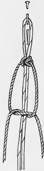
Second half ready to pull tight.
